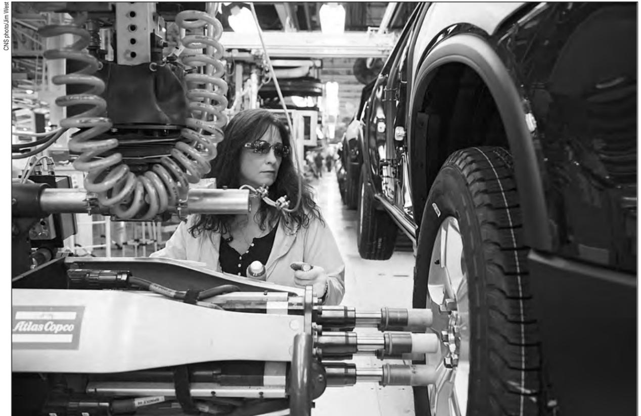
A worker tightens lug nuts on a wheel along an assembly line at a General Motors plant in Lansing, Mich., in 2008. The Second Vatican Council’s Dogmatic Constitution on the Church reaffirmed the ancient doctrine that all the faithful, no matter what their state in life, are called to “the fullness of the Christian life and to the perfection of charity.”
