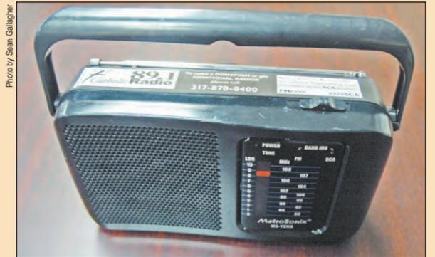
The "Small Miracle" radio allows people living within a 20-mile radius of Indianapolis to clearly receive Catholic Radio Indy 89.1 FM's broadcast on a sub-carrier signal.
